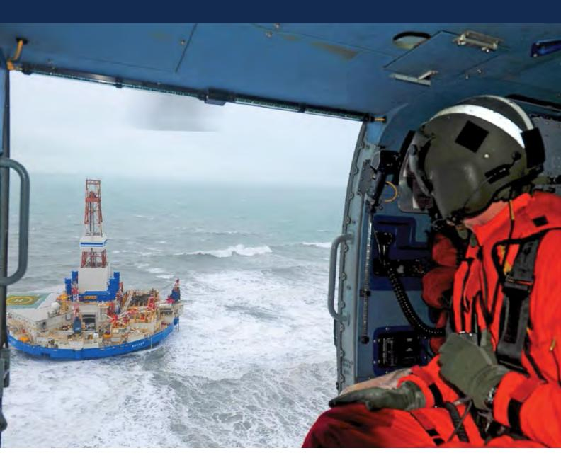
The Kulluk conical drilling unit, operated by Royal Dutch Shell, broke free from tow lines in heavy weather off Alaska and grounded on Sitkalidak Island in December 2012. The company had to shut down operations.
